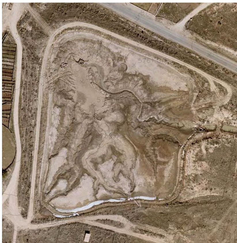
Figure 11. Mayfield Detention Pond (open channel influent on the right and outlet to pressurized pipe system on the upper left).
