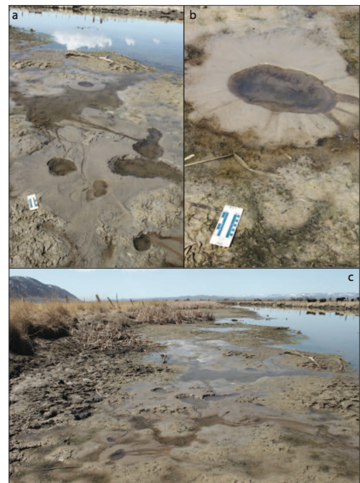
Figure 19. View of sand boil generated by liquefaction during the 2010 Mw 4.6 Randolph, Utah earthquake. Photo courtesy of Chris DuRoss, Utah Geological Survey.
