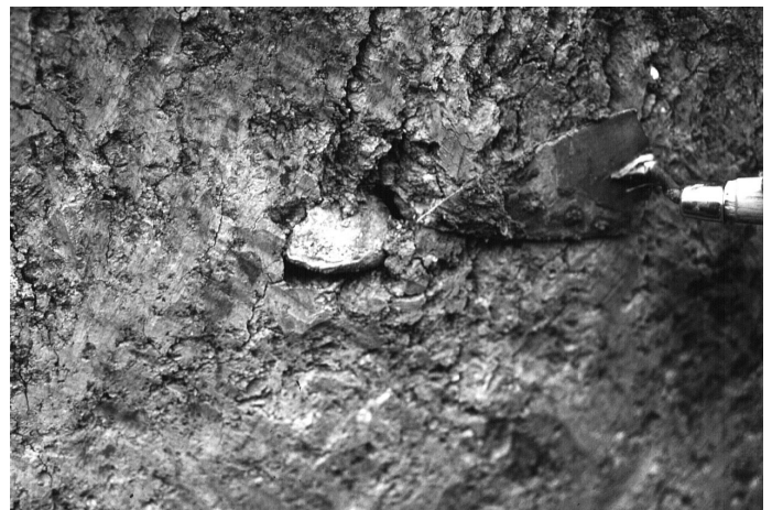
Figure 10. Harrisville trench flow-failure deposit (unit 2) containing subangular to subrounded gravel and cobbles.
