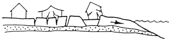
(e) Lateral Spreading and Resultant Pull-Apart Grabens
