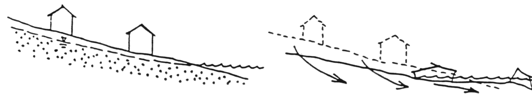
(c) Flow Failure
