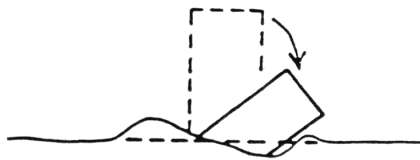
(e) Lateral Spreading and Resultant Pull-Apart Grabens
