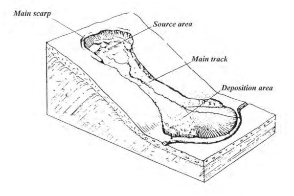
Attachment 2. Block diagram of features commonly associated with an earth flow (modified from Varnes, 1978).
