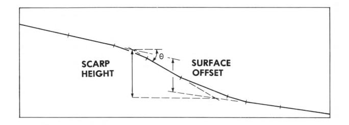
Figure 1.--Scarp profile showing definition of surface offset and scarp height. Tick marks on profile are the intervals measured in the field.  $\theta$  = scarp-slope angle.
