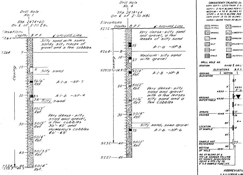
RELATIVE DENSITY(NON-PL. VERY LOOSE - LESS THAN 4 LOOSE - 4 TO 10 BLOWS PL MEDIUM - 10 TO 30 BLOWS PER DENSE- 30 TO 50 BLOWS PE VERY DENSE- MORE THAN 50 SOFT- 2 TO 4 BLOWS PER FO-MEDIUM - 4 TO 8 BLOWS PE STIFF- 8 TO 15 BLOWS PER VERY STIFF 15 TO 30 BLOWS DOLOWITE SANDSTONI SILTSTONE OFOO E ORLE ABBREVIATIO! L.L.- LIQUID LIMIT P.I -PLASTIC INC.
